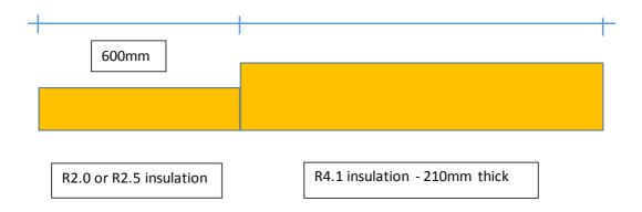
The perimeter insulation should not block off the air flow from the eave to the roof space.
