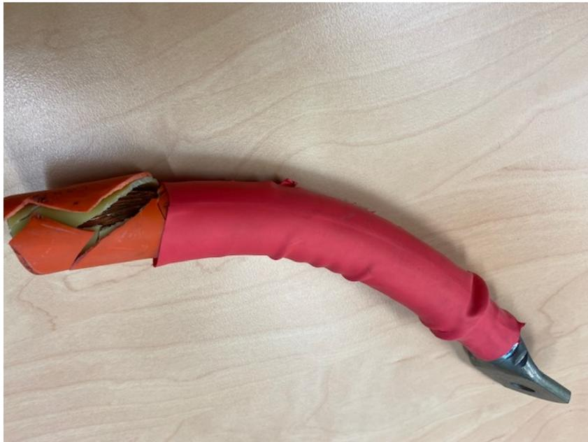
*Figure 1: Degraded cable found in Hobart*
