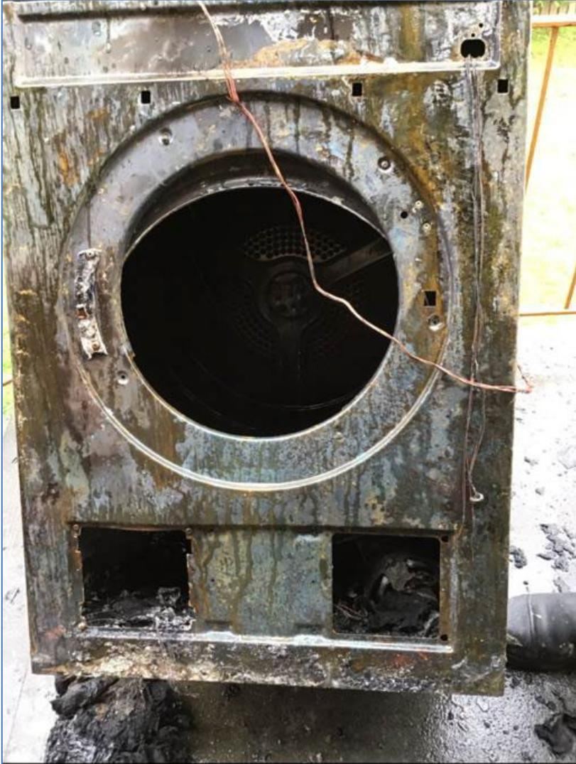
*Image 3: Fire damaged tumble dryer*
