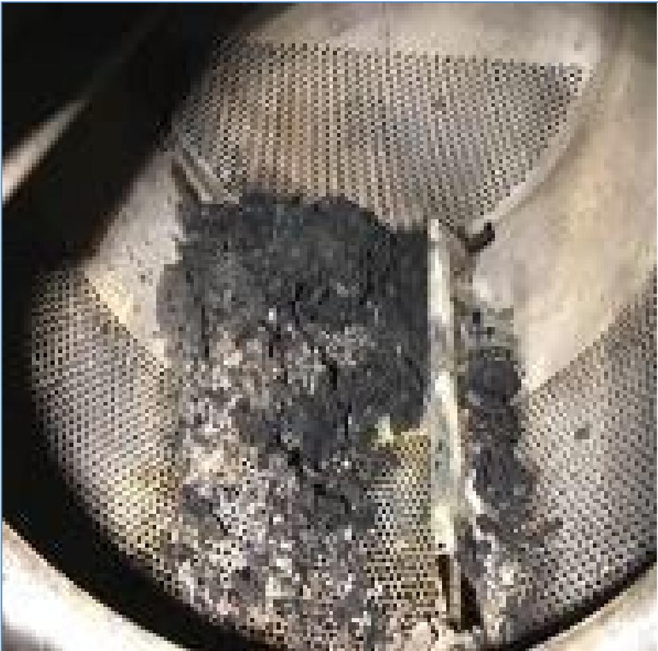
*Image 2: Fire damaged contents inside a tumble dryer*
